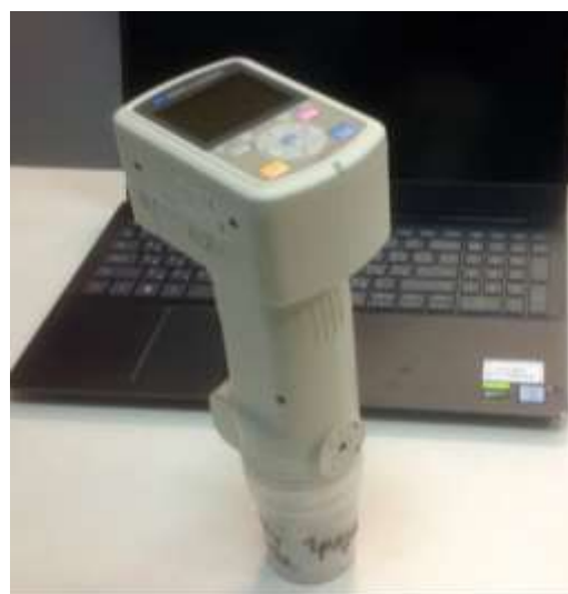
Figure 5. Portable spectrophotometer CM-600d (Japan) for determination of whiteness and yellowness of soda-sulphate mixture.
